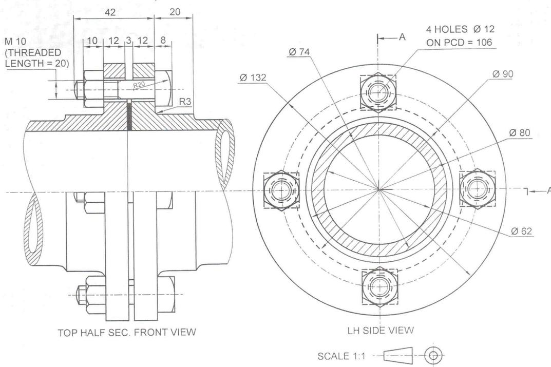
ASSEMBLY OF A FLANGED PIPE JOINT
